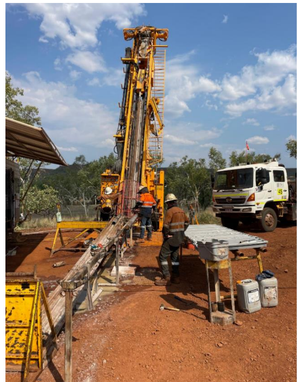
Diamond drilling in progress
