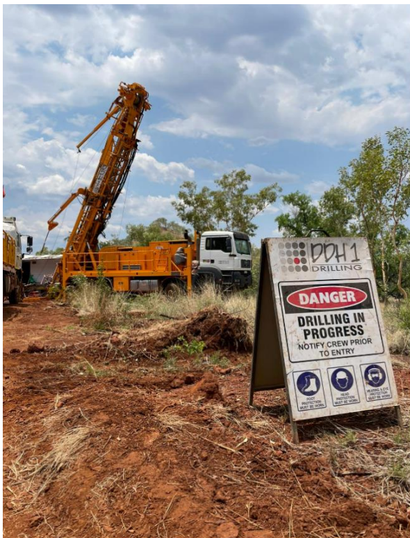
Diamond drilling in progress
